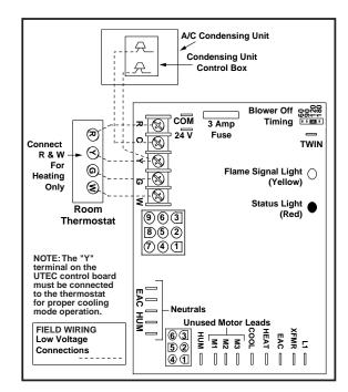
Figure 28. Low Voltage Field, Four-wire Heating/Cooling Applications
